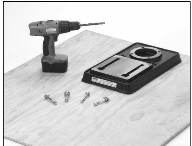
Figure 3. Attaching plywood sub-base.
